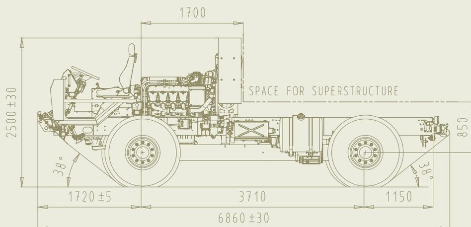
The TATRA 4x4 High Mobility Heavy Duty (HMHD) chassis is built as a platform for various kinds of special vehicles that need: • superior drive ability in difficult terrain • heavy armoured protection on top of the chassis • reliable chassis with low life cycle costs
