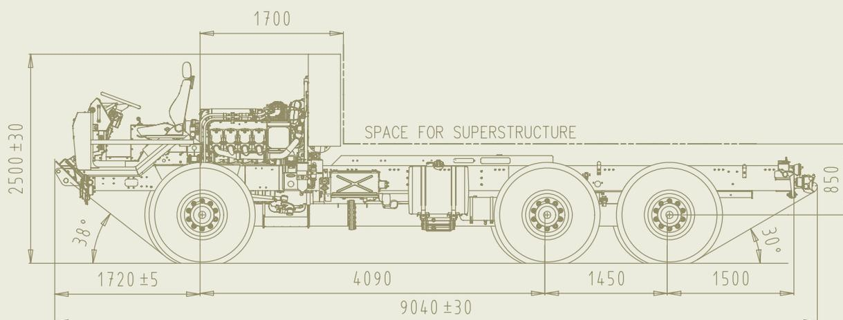
The TATRA 6x6 High Mobility Heavy Duty (HMHD) chassis is built as a platform for various kinds of special vehicles that need: • superior drive ability in difficult terrain • heavy armoured protection on top of the chassis • reliable chassis with low life cycle costs
