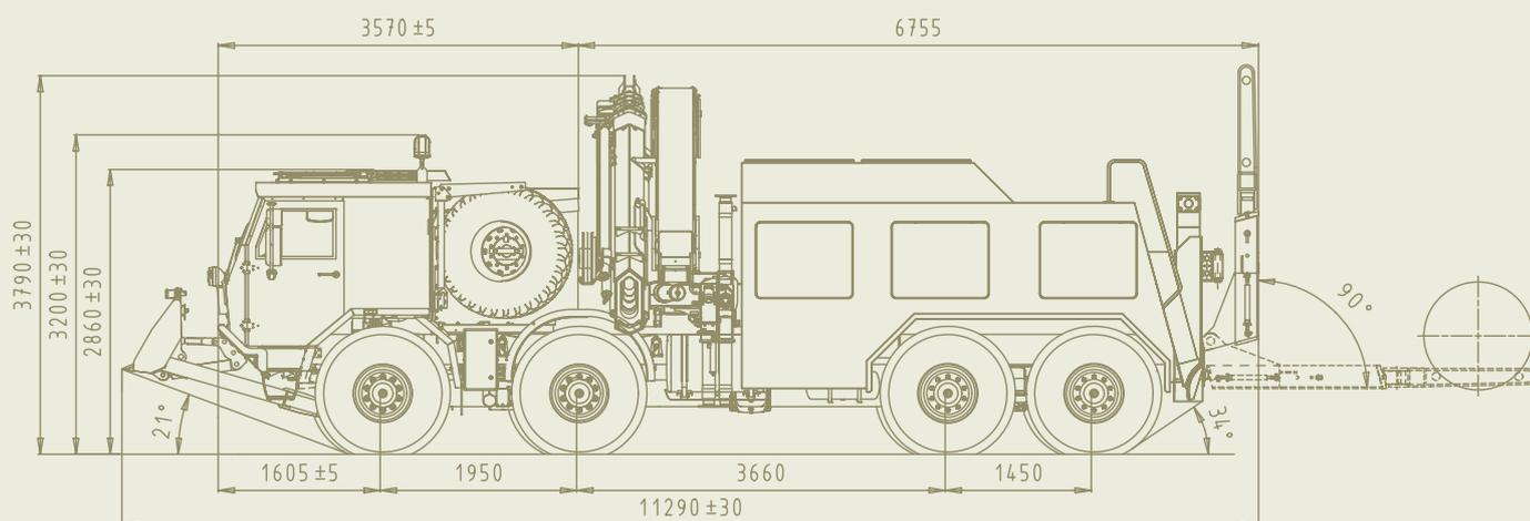
The High Mobility Heavy Duty (HMHD) Recovery Vehicle is able to recover armoured vehicles very quickly and efficiently in a tactical environment. The vehicle capability and payload enabling to recover heavy armoured vehicles and it is capable of towing most types of current and future wheeled vehicle systems and their variants. The vehicle is able to overturn crashed vehicles, perform slope recovery and make an access to unapproachable places.
