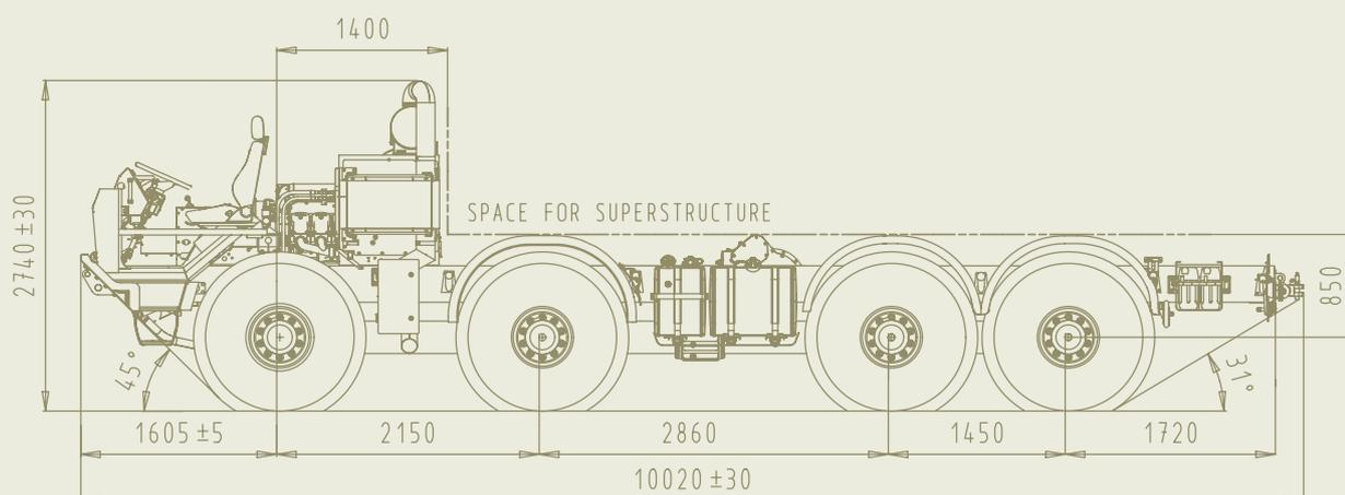
The TATRA 8x8 High Mobility Heavy Duty (HMHD) chassis is built as a platform for various kinds of special vehicles that need: • superior drive ability in difficult terrain • transport troops or sensitive material over difficult terrain • heavy armoured protection on the chassis • reliable chassis with low life cycle costs
