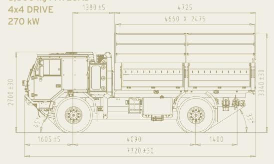
me, which are unique characteristics of the TATRA concept chassis proven for more than 90 years. It allows each wheel to move independently, with improved steering, and maximum tire-to-ground contact, while featuring extrethe backbone tube with a conventional ladder frame via several cross-members. In addition, the backbone tube
