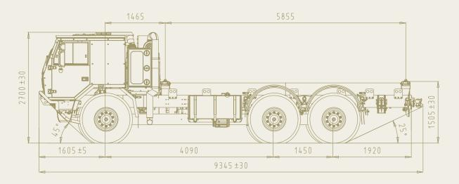
try conditions. It can serve as a tactical truck, or carry various kinds of special superstructures and load handling systems. Exceptional resistance of the chassis against twist and bending, as well as low transfer of vibrations on the load make it ideal means for transporting standard containers and shelters, sophisticated electronics, or other
