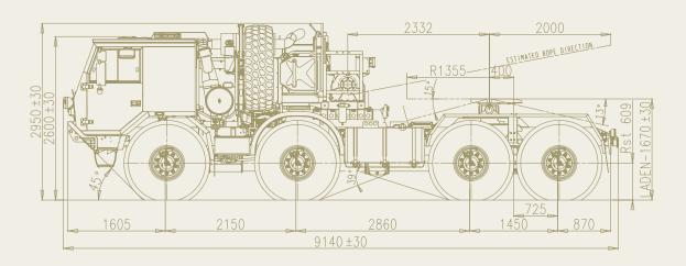
The TATRA Tank Transporter (TTT), 8x8 high mobility heavy duty (HMHD) semitrailer prime mover comes from the FORCE family, range of heavy tactical wheeled vehicles.
