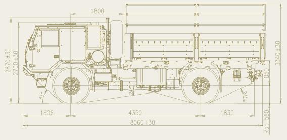
me, which are unique characteristics of the TATRA concept chassis proven for more than 90 years. It allows each wheel to move independently, with improved steering, and maximum tire-to-ground contact, while featuring extreme resistance of the chassis against torsion and bending. This is provided by a solid 3D frame formed by connecting the backbone tube with a conventional ladder frame via several cross-members. In addition, the backbone tube
