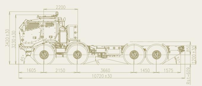
The TATRA 8x8 High Mobility Heavy Duty Tactical Truck is a member of the TATRA FORCE family, heavy-duty vehicles designed for rough terrain, difficult climatic and environment conditions. The 8x8 all-wheel drive chassis employs
