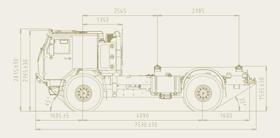
me, which are unique characteristics of the TATRA concept chassis proven for more than 90 years. It allows each wheel to move independently, with improved steering, and maximum tire-to-ground contact, while featuring extrethe backbone tube with a conventional ladder frame via several cross-members. In addition, the backbone tube
