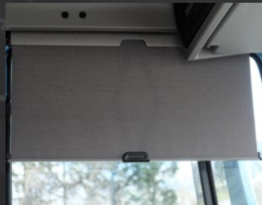
Retractable side blinds on the driver and front passenger side.
