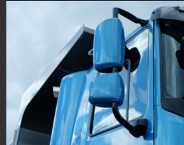
Electronically operated twin mirrors in the cab colour.
