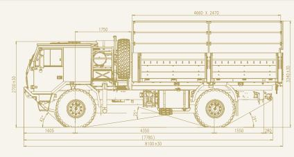
INDEPENDENT SUSPENSION SOLID 3D STRUCTURE FRAME 8,500 kg PAYLOAD 4×4 DRIVE 257 kW
