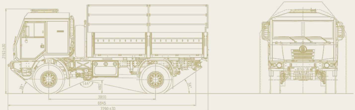
**The new TACTIC family vehicle is a further development of the successful T810 model, the TATRA medium-class, all-wheel-drive, off-road logistic truck designed to carry different superstructures up to 5.5t of total payload.**
