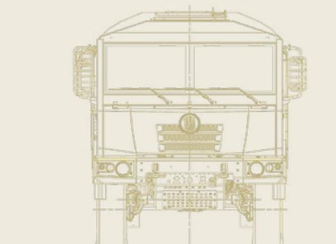
The new TACTIC family vehicle is a further development of the successful T810 model, the TATRA medium-class, all-wheel-drive, off-road logistic truck designed to carry different superstructures up to 5.5 t of total payload.
