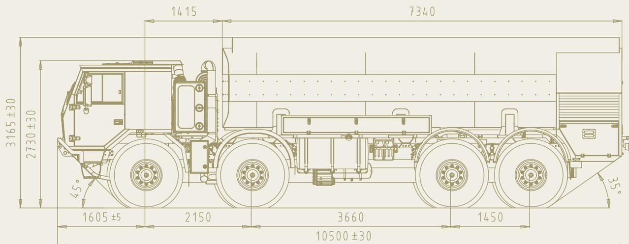
The TATRA 8x8 fuel tanker is suitable for operation in the most difficult off-road or cross-country conditions. The vehicle can be used for transporting of fuel to different reservoirs or for direct filling of smaller refuelling tankers. Design and equipment according international standard for transporting of danger liquid - ADR - code LGBF and other STANAG standards.
