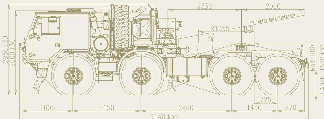
The TATRA Tank Transporter (TTT), 8x8 high mobility heavy duty (HMHD) semitrailer prime mover comes from the FORCE family, range of heavy tactical wheeled vehicles.
