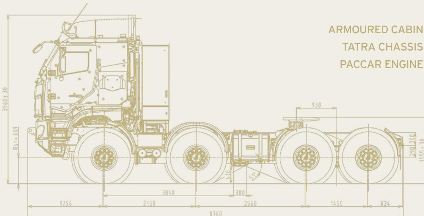
The heavy-duty TATRA PHOENIX tractor with 8x8 all-wheel drive uses a combination of independently suspended semi-axles, a backbone frame and modern Paccar engines.
