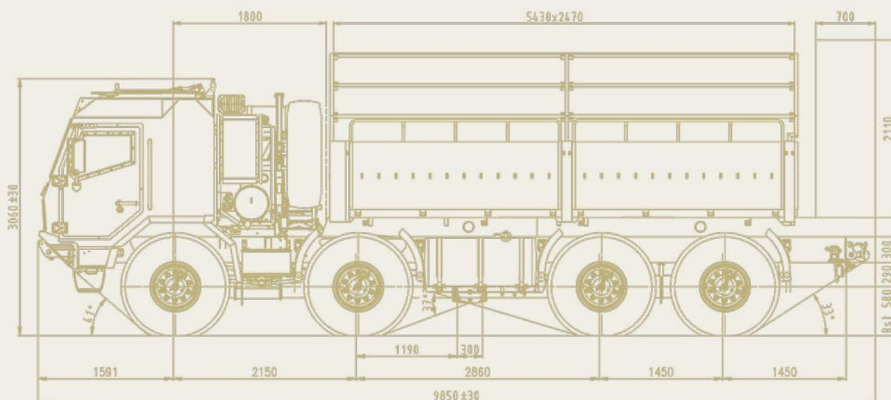
**The 8x8 ammunition carrier is designed for high mobility operations in very difficult terrain and climatic conditions. The unique TATRA backbone tube chassis gives excellent mobility at low Life Cycle Cost.**
