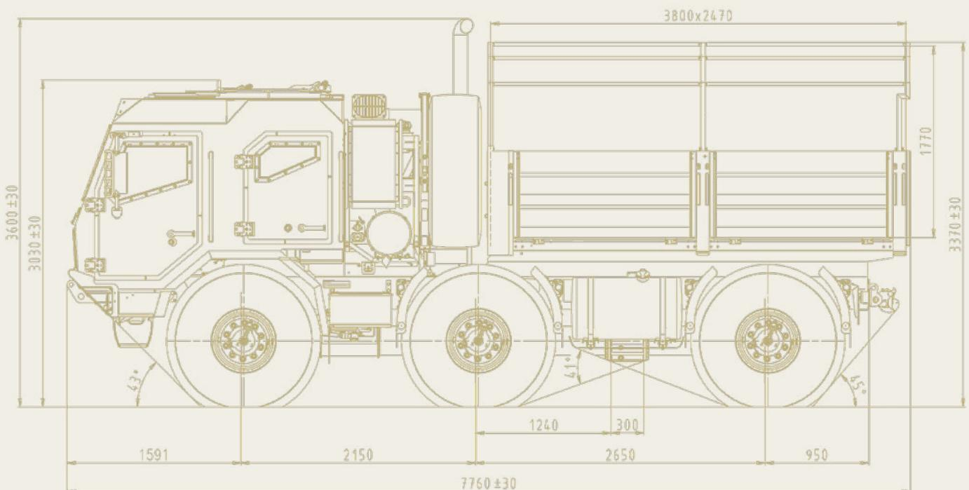
The 6x6 cargo/troop carrier is designed for high mobility operations in very difficult terrain and climatic conditions. The unique TATRA backbone tube chassis gives excellent mobility at low Life Cycle Cost.
