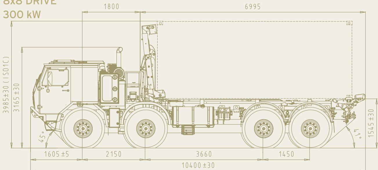
The TATRA 8x8 High Mobility Heavy Duty (HMHD) Tactical Truck integrated with military Load Handling System interfaces with NATO STANAG 2413 flatracks, bodies and existing in-service military flatracks and bodies (even with non-standard side rails). System installed height with ISO1C container is minimised under 4m to meet European road regulations.
