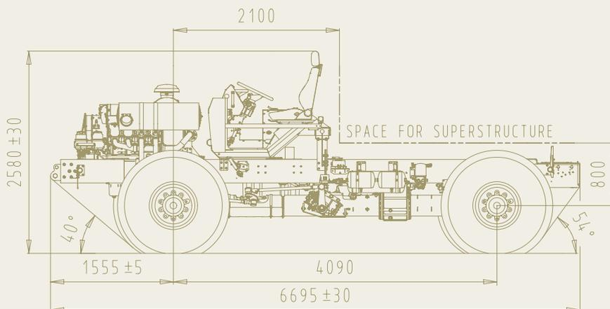
The TATRA 4x4 High Mobility Heavy Duty (HMHD) chassis is built as a platform for various kinds of special vehicles that need: • superior drive ability in difficult terrain • heavy armoured protection on top of the chassis • reliable chassis with low life cycle costs
